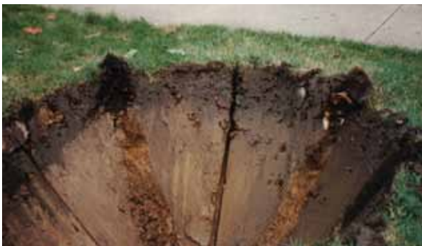
Photograph 2B-3. Soils on parkways typically have high clay content as shown below the dark topsoil layer in the planting hole. The clay limits to some degree the palate of tree species that can successfully be used in the Village.
