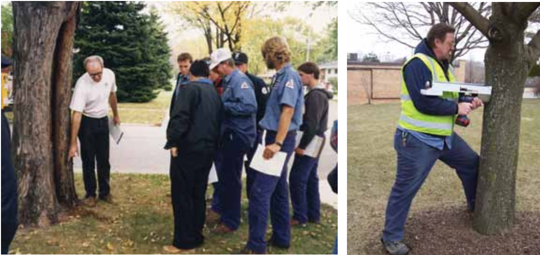
Photograph 3H-1a and 1b. Left: The Village has done extensive training on tree risk evaluation for Forestry staff and crews. Right: Close evaluation and testing of potential risk trees is conducted annually by the Village. The tree is being tested for decay using a Resistograph™
