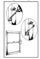
lower window and partially into the frame of the upper window. Insert the "pin" (nail, eye bolt, or dowel rod). The window cannot be opened until you remove the pin. A second set of holes allows the window to be partially opened (about 4 or 5 inches) and locked to allow ventilation. You may also purchase special key locks for windows at hardware stores.
