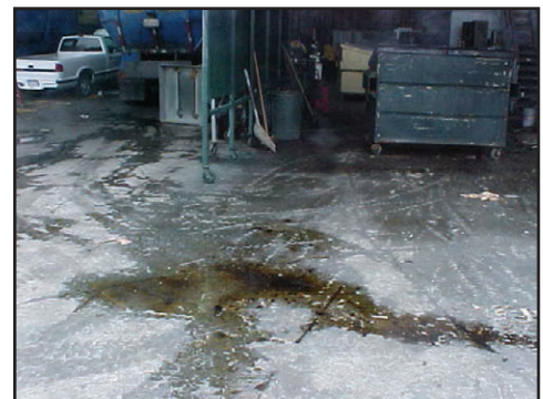
Figure 16. Good housekeeping is probably the most common BMP in SWPPPs. Poor sweeping practices can contribute significant pollutants in stormwater runoff.
